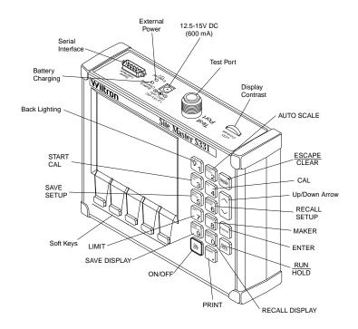
Figure 2-1. Site Master Controls and Connectors
